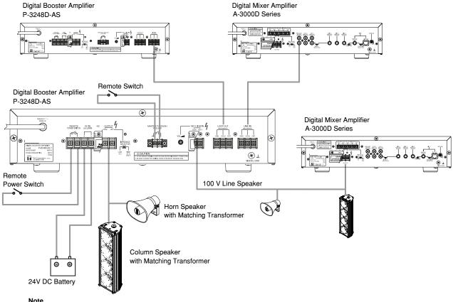
Use battery with current capacity minimum 40 Amperes.
