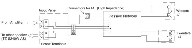
Note: Screw terminals is connected parallel internally
