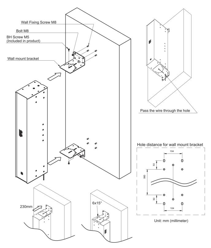
Note: Bolt and screw for wall is not provided. Please use bolt and screw which suitable with wall structure and able to handle weight of units.
